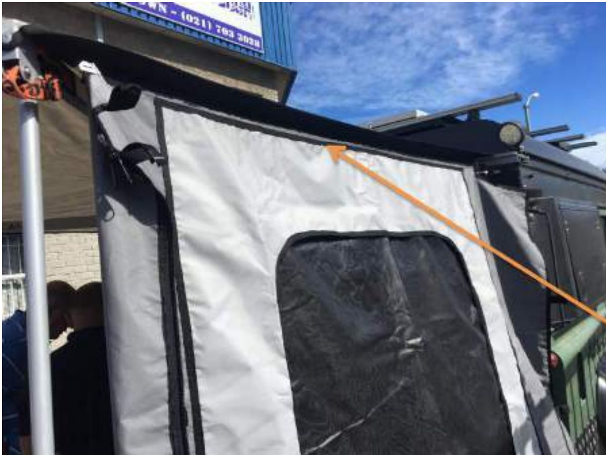
Figure 13: Awning Side 1 attached using Top Velcro
