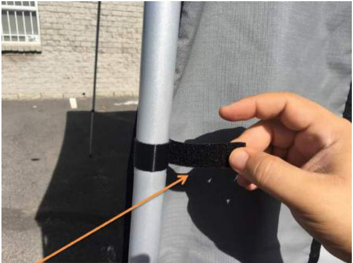
Figure 14: Velcro Straps on the Awning Sides Canvas
