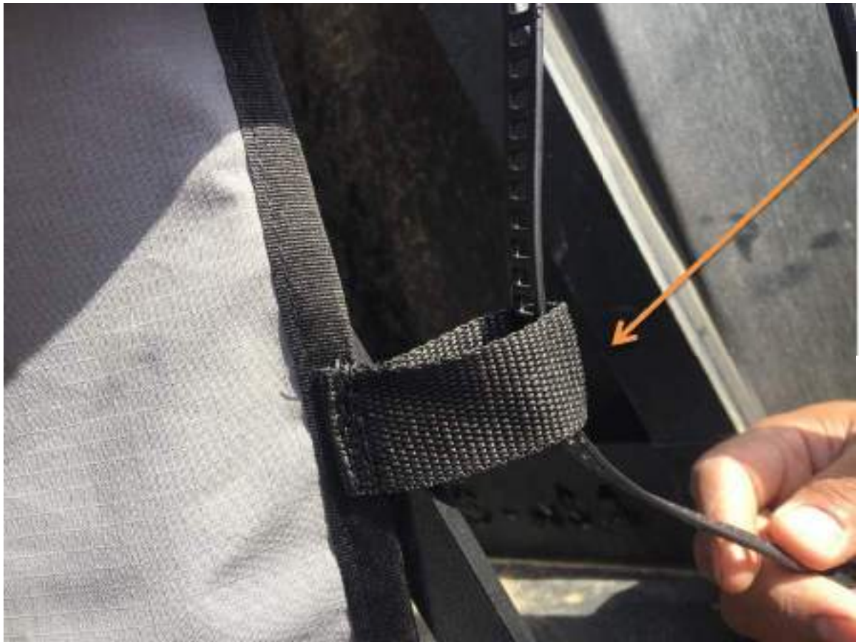
Figure 17: Flexi Tie threaded through Canvas Loop
