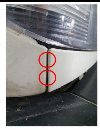
First remove lower panel using a thin driver at the circiled points
