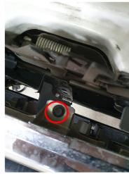
Remove Grille by unscrewing the bolts securing it
