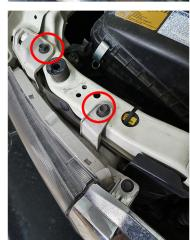
Remove each Headlight by unscrewing 4 bolts securing it
